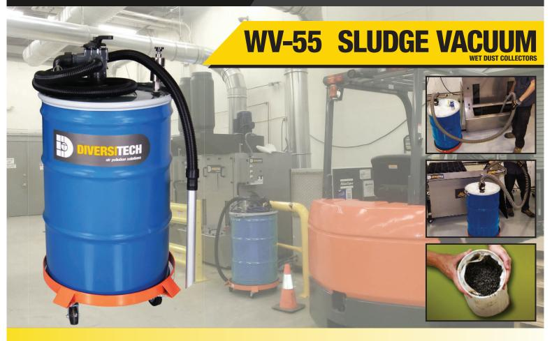
The WV-55 sludge vacuum offers a fast, easy way to clean dust, chips and swarf out of wet dust collectors and other equipment. The WV-55 vacuums water along with the sludge and collects the solids in a reusable 5 micron filter bag. The vacuum can then pump back out only the water for reuse in the wet collector. The sludge vac is ideal for use on machines with sumps, parts washers or any storage containers with contaminated liquids and reduces manual maintenance requirements.
