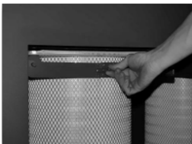
2. Unhook barrel bolt latch.
