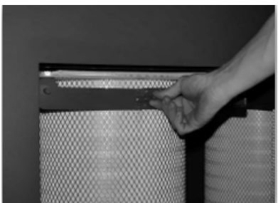
7. Hook barrel bolt latch.
