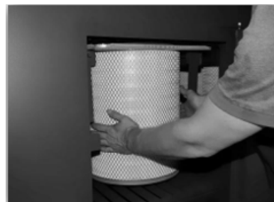
6. Insert clean replacement filter.
